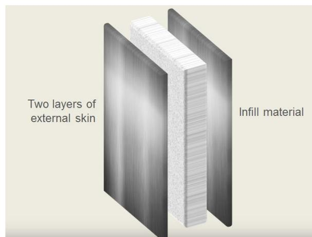
Figure 3. A typical insulated panel comprising two tough external faces, usually metal, and a high performance internal insulant core.
