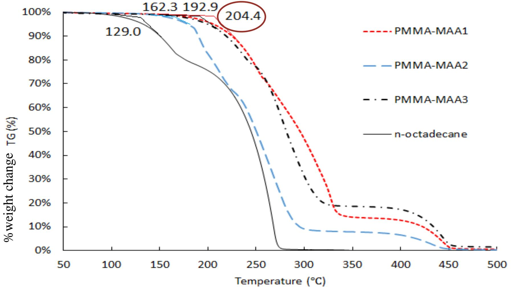
TGA curves of MEPCM samples: % weight change as a function of temperature
